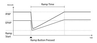
If ramp is activated with AVAPS enabled, it will reduce the maximum pressure support capability to IPAP Min or PS Min and ramp to the IPAP Max or PS Max over the ramp time period. During the ramp period, the prescribed tidal volume may not be acheived.
