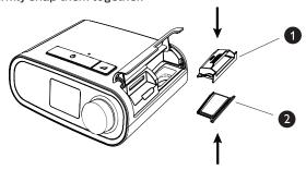
3. Place the new filter assembly back in the side of the therapy device. Swing the door closed.
